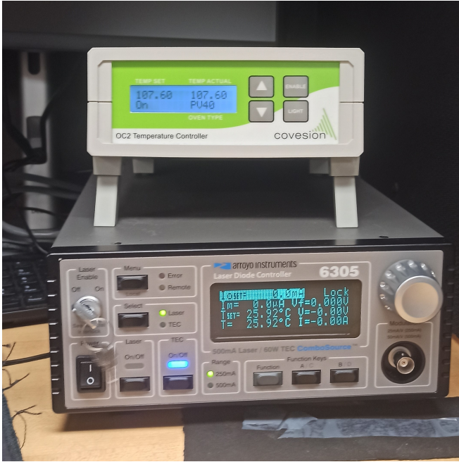
FIG. 3: Oven temperature controller (top) and laser temperature and current controller (bottom).
